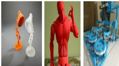
Fig.2. Objects produced using FDM and SLS Technology from plastics and alumide materials (figures are only for illustrative purpose).
